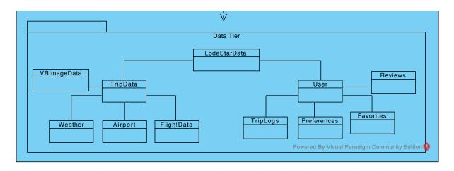
Figure 9 - Data Tier Subsystem of Server
