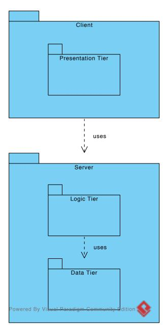
Figure 1 - Subsystem Decomposition
