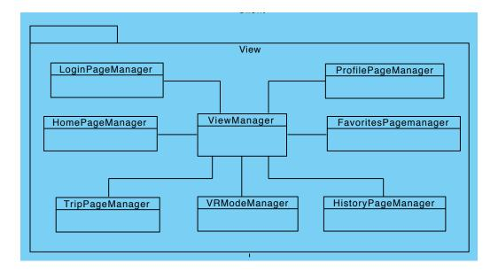
Figure 6 - View Subsystem in Client
